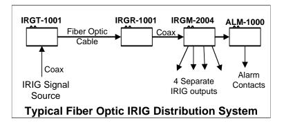
The IRGM-2004 provides four electrical outputs. Multiple IRGM-2004 units may be "daisy-chained" when more than 4 output channels are required.
