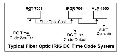
Both should be connected as shown and a DC time code signal applied to the transmitter. The receiver will reproduce this signal with no adjustments.
