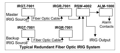
Upon loss of the primary IRIG signal, the RSW-4002 will automatically switch the remaining secondary (backup) IRIG signal to the output as well as activate the front panel alarm indicator and ALM-1000 Alarm Sensing Unit if used.
